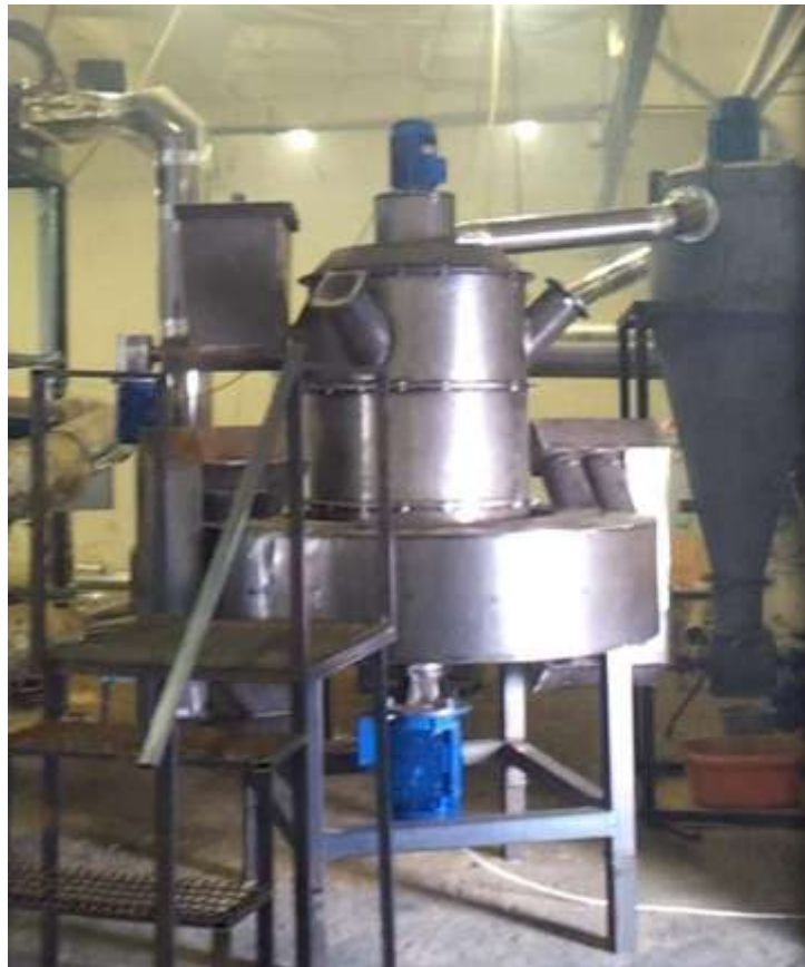
Fig.4. Vortex and cyclone dryer of the demonstration plant
