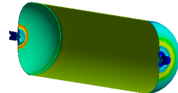
Von Mises Stresses under 500bar Pressure
