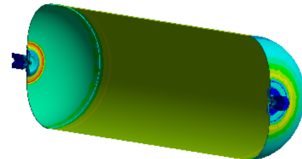
Von Mises Stresses under 500bar Pressure
