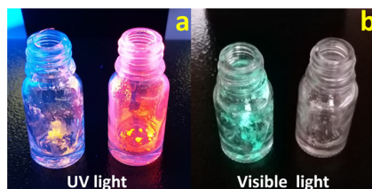
Figure 1. Photoluminescent ink (a) under UV–vis light and (b) under visible light; UV light is switched off. In this concept, the dual emission is clearly visible and only one excitation of light at 325 nm is employed without the need for near-infrared laser excitation light (photo taken by O.M.).
