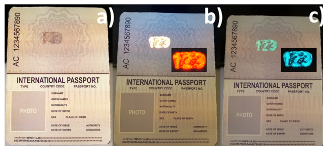
Figure 5. 123 numbers screen with the anti-counterfeiting photo-luminescent ink of \text{Eu}(\text{FAC})_3\text{Phen} , \text{SrAl}_2\text{O}_4:\text{Eu} , Dy, and PVB added on top of the passport's image showing a dual-mode emission effect under similar UV excitation wavelength. (a) Composite under normal light, (b) under UV light, red emission is clear, and (c) green afterglow luminescence persisted, lasting for a few minutes, upon removal of the UV light (photo taken by O.M.).
