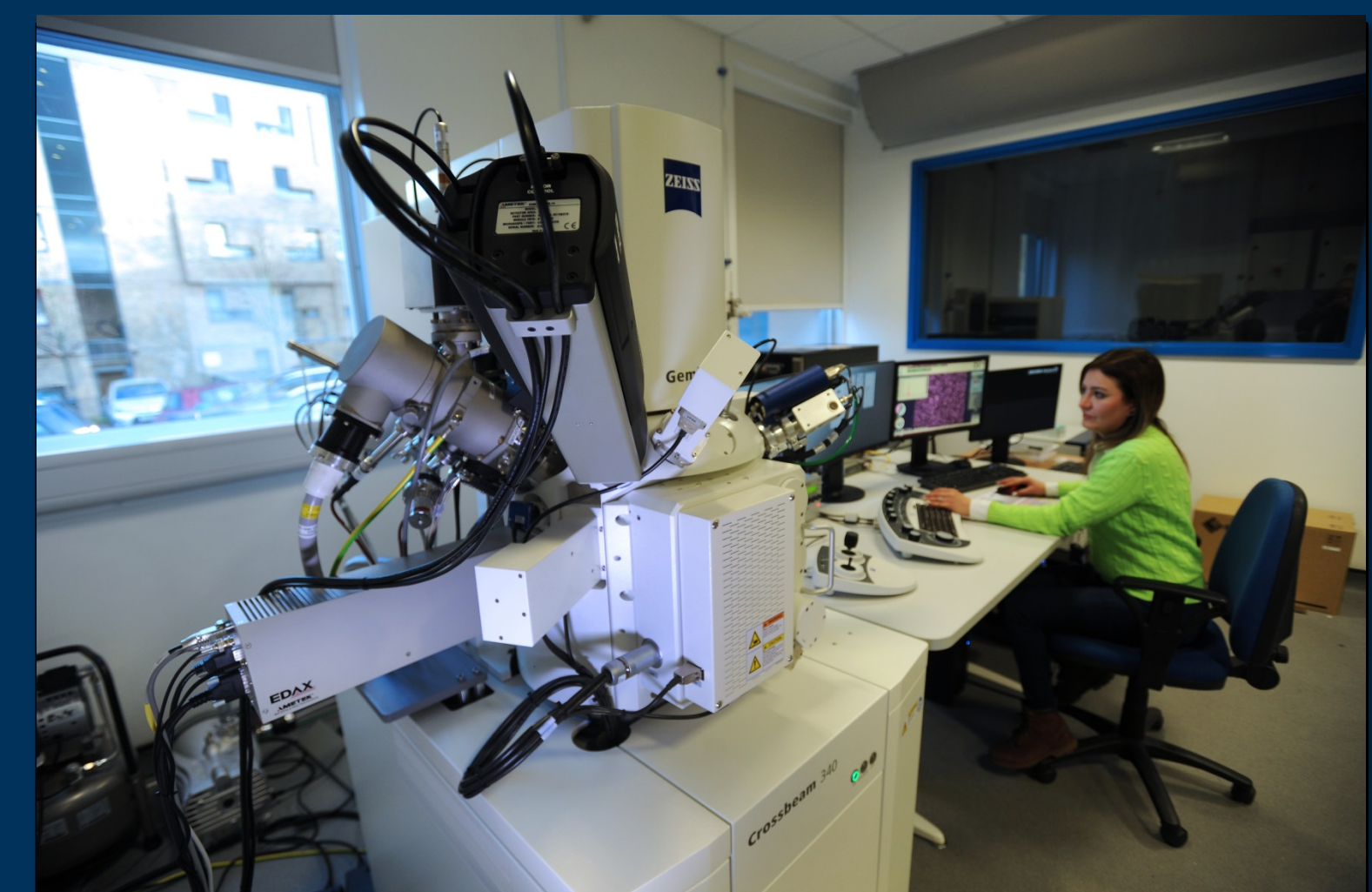
Focused Ion Beam SEM, equipped with EDAX Octane Elite SDD EDX and EBSD
