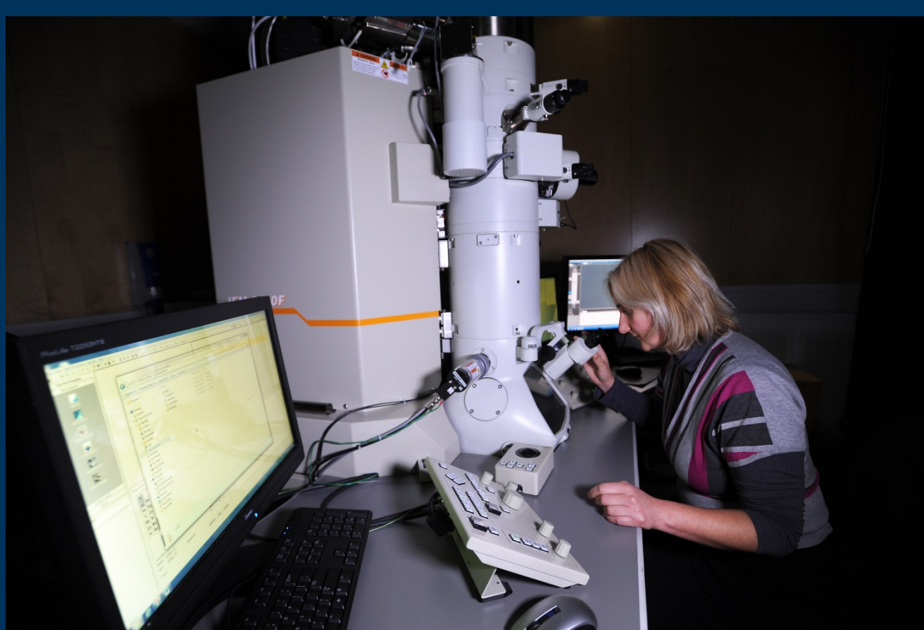
Transmission Electron Microscopy, equipped with X-ray, electron energy loss spectrometry and cathodoluminescence.
