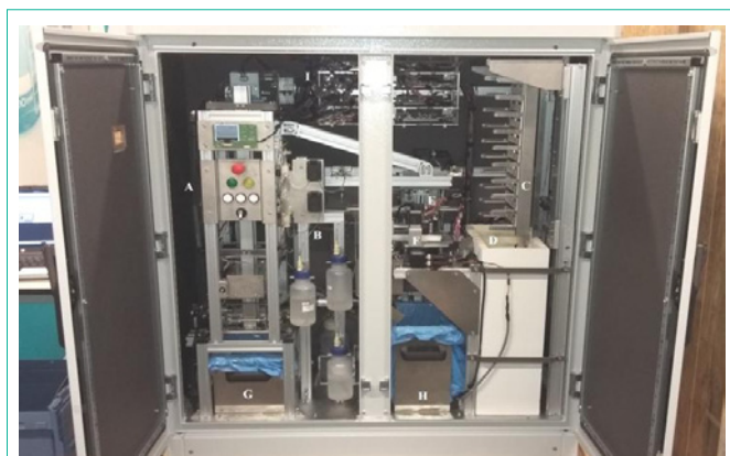
Figure 1: Automated analyzer consisting of: A) Filtering module, B) Elution and washing zone, C) Cartridge dispenser, D) Fridge, E) Analytical module, F) Telescopic handler, G) Container of used filters, H) Container of used cartridges, I) Electric control panel.
