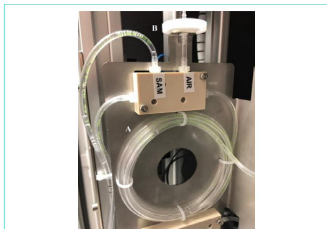
Figure 3: Nine milliliter-sample loop consisting of: A) tygon tubing loop; B) PTFE Filter membrane pore size 0.2 \mu m.
