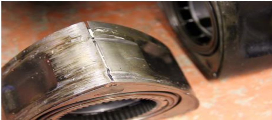
Figure 6 Damaged rotor of Wankel engine
