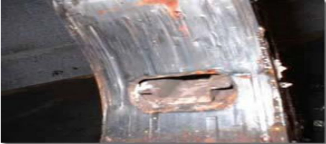
Figure 7 Damaged rotor-housing of Wankel engine
